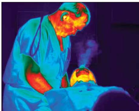
Figure 1: Visualization of nitrous oxide (N<sub>2</sub>O) from the patient's breathing zone in a dental operator.
