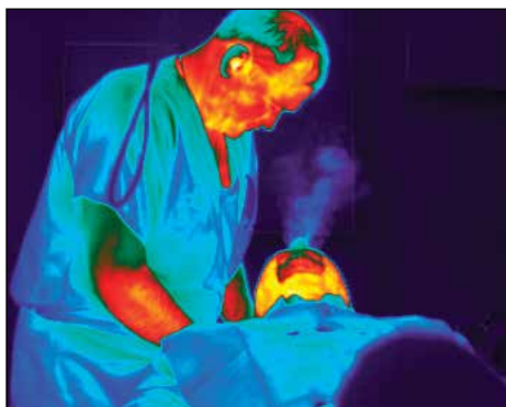
Figure 1: Visualization of nitrous oxide (N 2 O) from the patient's breathing zone in a dental operator.
